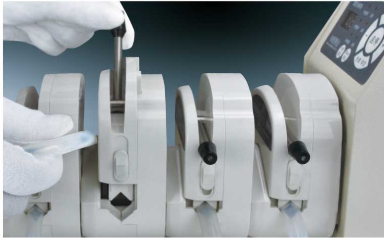
Mounting several pump heads can increase the flow rates
